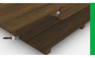
Before installing the product, the head parts should be sealed (whether or not end-matching is preferred) to prevent moisture absorption. Thus, end-splits that may occur are minimized.
