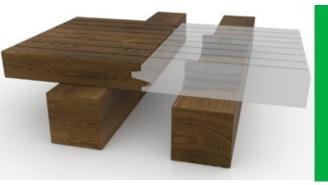
Whether with end-matching or not deck finishes do not have to be laid on underconstruction.
