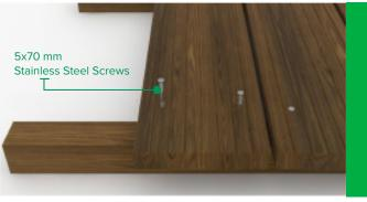
In mount face screwed decking applications 5x70 mm stainless steel screws with high torsion should be used.
