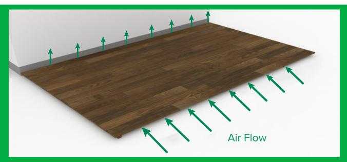
In order to keep the wood dry continuously and prevent water accumulation below the decking area, it is necessary to provide the necessary distance for air circulation.
