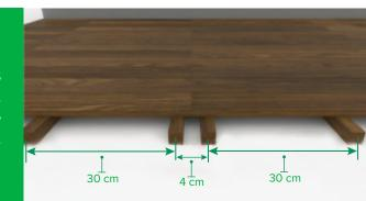
5 mm distance should be left between decking and underconstruction to avoid contact. With Tantak System clips, this distance is given automatically. With this method, air circulation will be provided and the moisture absorption is reduced to a minimum.
