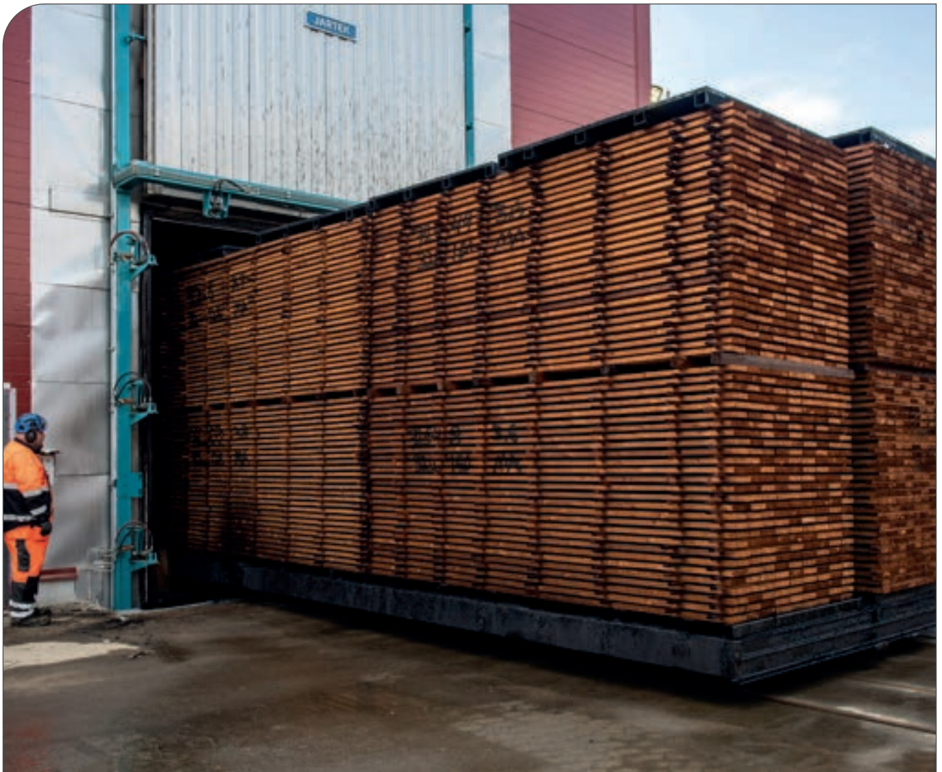
Figure 4. ThermoWood® being manufactured in process kiln.
